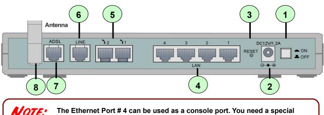
The Ethernet Port # 4 can be used as a console port. You need a special console tool which already includes in the package to connect with LAN port 4 and PC's RS-232 port (9-pin serial port).
