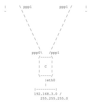
We have three routers A, B and C. Each router supports one ethernet segment with a Class C IP network (netmask 255.255.255.0). Each one also has a PPP link to each of tEthernet routers. The network ultimately forms a triangle.
