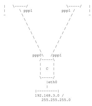
We have three routers A, B and C. Each supports one ethernet segment with a Class C IP network (netmask 255.255.255.0). Each router also has a PPP link to each of the other routers. The network forms a triangle.
