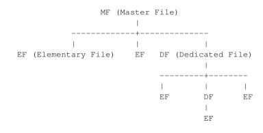
MF (Master File), can be seen as the root directory where the headers of elementary files and dedicated files are contained. Dedicated files are like the ordinary directories and elementary files are just data files. The PIN is also stored in an EF but only the card has access permission to this file. The attributes of the files on UNIX environments are changed to access conditions. Many cards have access condition lists which must be fulfilled before accessing the data.
