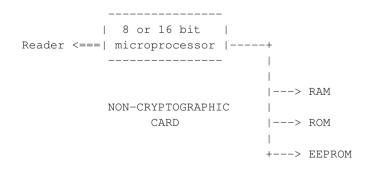
As seen in the diagram above all communication is done over the microprocessor, There is no direct connection between the memory and the contacts. The operating system is responsible for the security of the data in memory because the access conditions are controlled by the OS.
