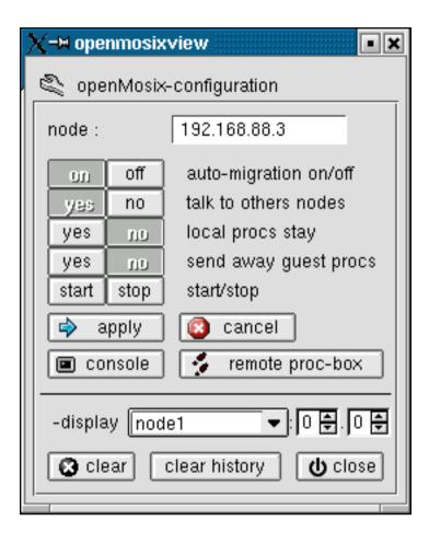
The openMosix-configuration of each host can be changed easily now. All commands will be executed per "rsh" or "ssh" on the remote hosts (even on the local node) so "root" has to "rsh" (or "ssh") to each host in the cluster without prompting for a password (it is well described in a Beowulf documentation or on the HOWTO on this page how to configure it).
